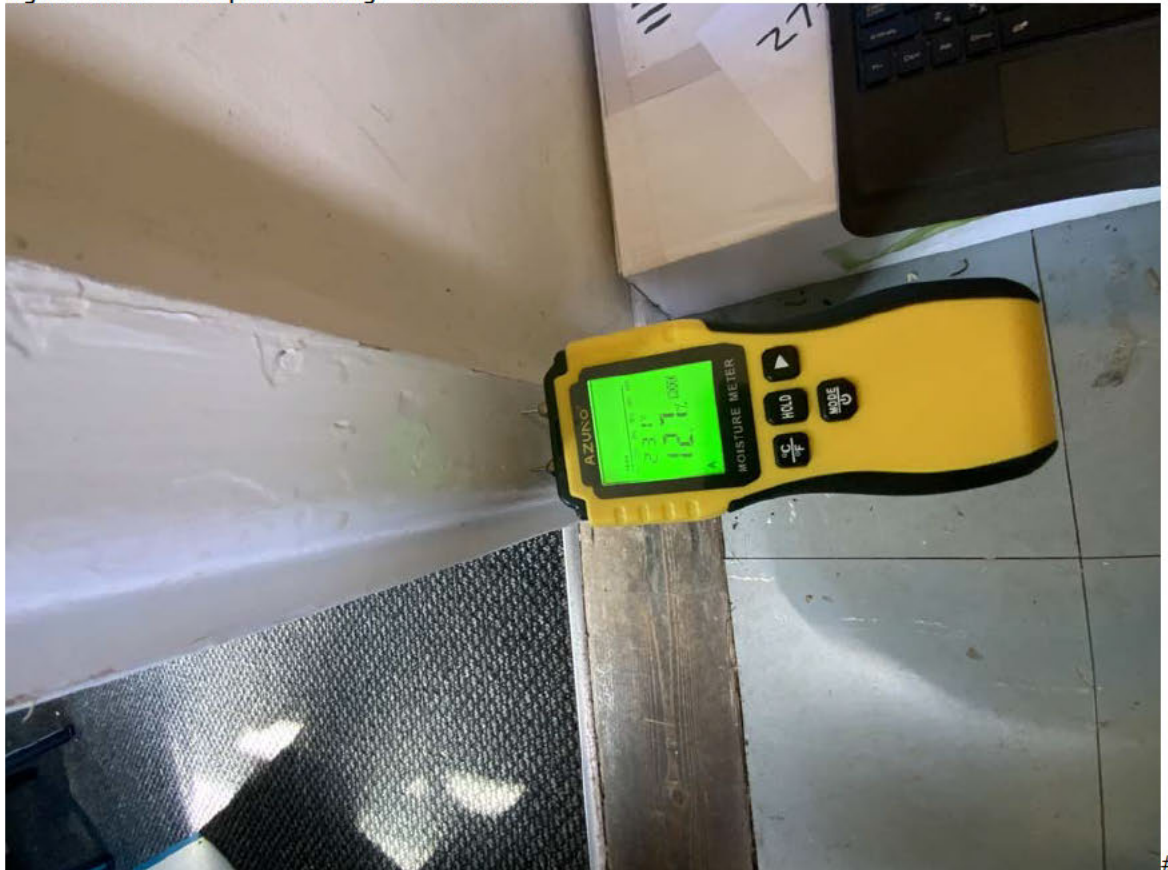
Figure 116.20 – Dampness readings (significantly damp area shown here for floor of main entrance)
