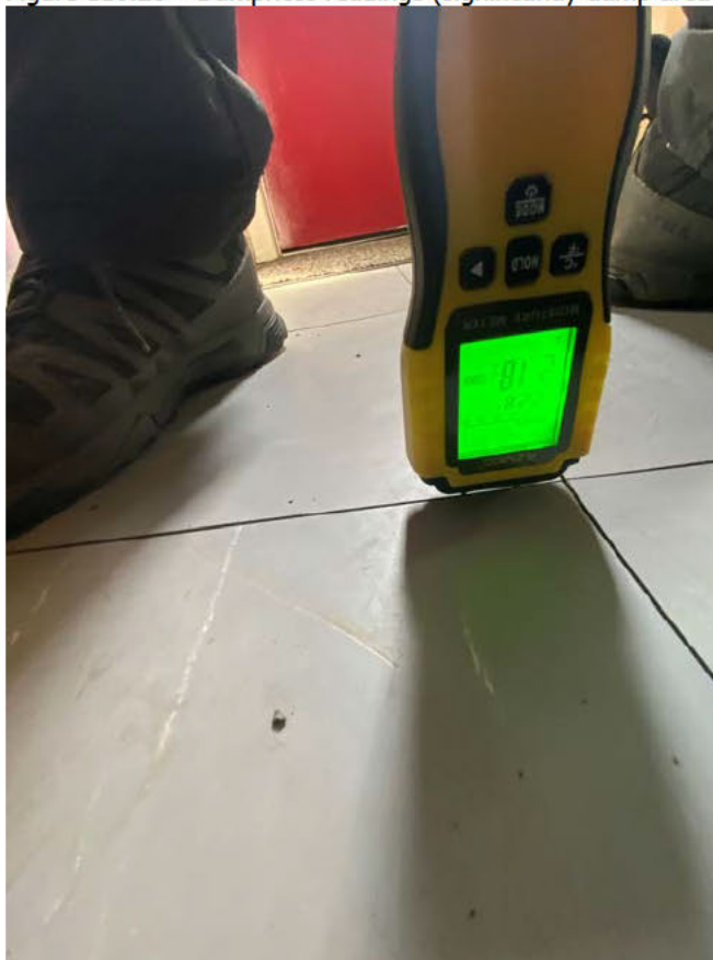
Figure 116.20 – Dampness readings (significantly damp area shown here for floor of main entrance)
